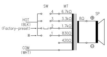
When oprating the speaker on 100 V line, do not set the impedance selection switch to this position.
